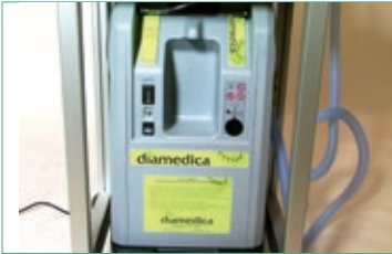
The Oxygen Concentrator provides both oxygen and air through the flowmeters on the control panel.
