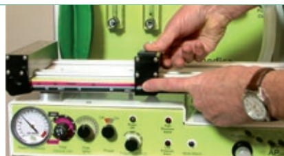
Patient pressure controlled by moving weights
