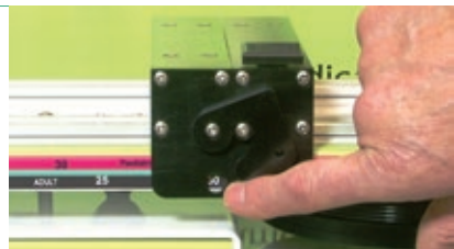
Patient pressure controlled by moving weights
